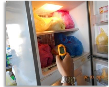
(b, c) Improper storage of raw foods in the refrigerator and temperature tested to be higher than the acceptable standard
